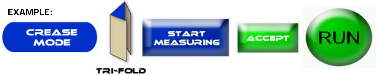
**Z Fold:** Press the Crease Mode Button > Z Fold > Start Measuring > Physically Run a sheet through the machine for the sensor to measure > Accept > Run.
