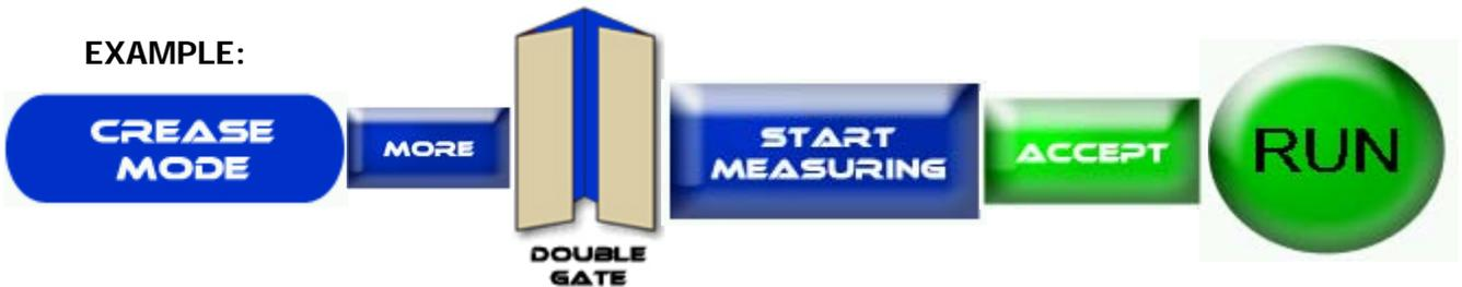
**Double Parallel Fold:** Press the Crease Mode Button > More > Double Parallel > Start Measuring > Physically Run a sheet through the machine for the sensor to measure > Accept > Run.
