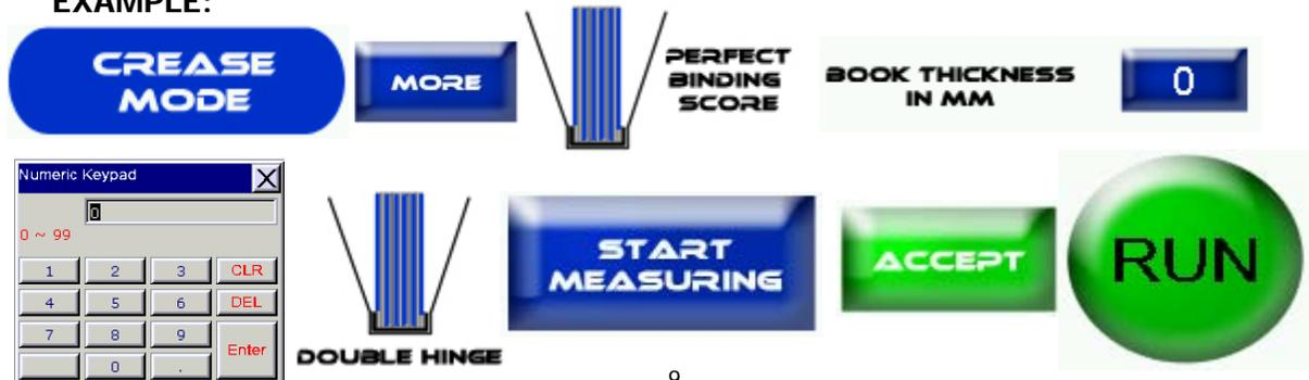
**Perfect Bind Single Hinge:** Press the Crease Mode Button > More > Perfect Binding Score > Enter The Book Thickness > Single Hinge > Start Measuring > Physically Run a sheet through the machine for the sensor to measure > Accept > Run.
