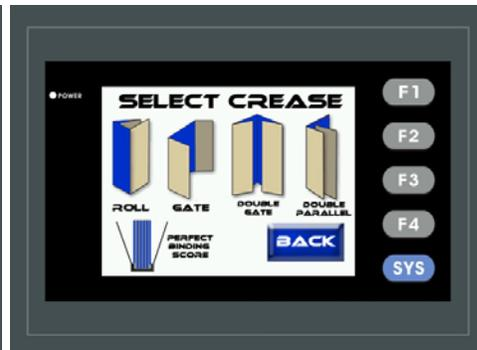
Crease selections include half, tri-fold, z fold, letter fold, roll fold, gate fold, double gate, double parallel, 3 perfect bind selections and 12 custom crease locations.
