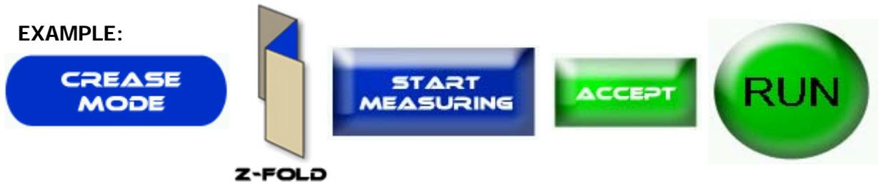
**Letter Fold:** Press the Crease Mode Button > Letter > Start Measuring > Physically Run a sheet through the machine for the sensor to measure > Accept > Run.
