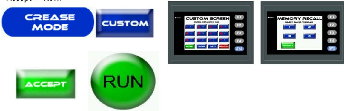
**Micro Adjusting the Crease Position:** Press the adjust button from the run screen. You can micro adjust each crease by pressing the arrow keys each direction. Each press will adjust by 1/13th of a mm. Each Adjustment is relative to the one before it so if you adjust crease 1 by 3 clicks it will also move all the creases after it. You would then need to adjust them back 3 clicks each.
