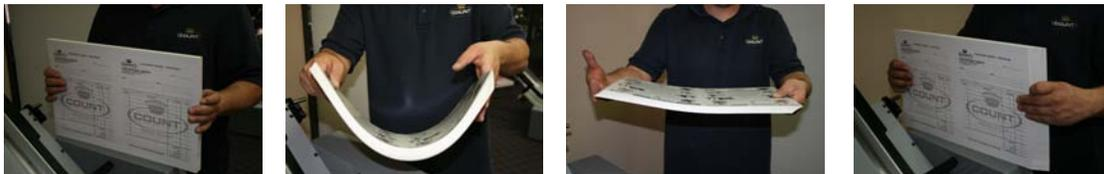
As seen above take a stack in-between 1-3 inches and hold it straight. Next fold the stack inward, hold tight on your right hand and loose on your left then hold tight on your right hand and loose on your left and straighten the stack back out. Gently tap the stack on the side cover to ensure alignment and load the stack in the feeder as seen below.
