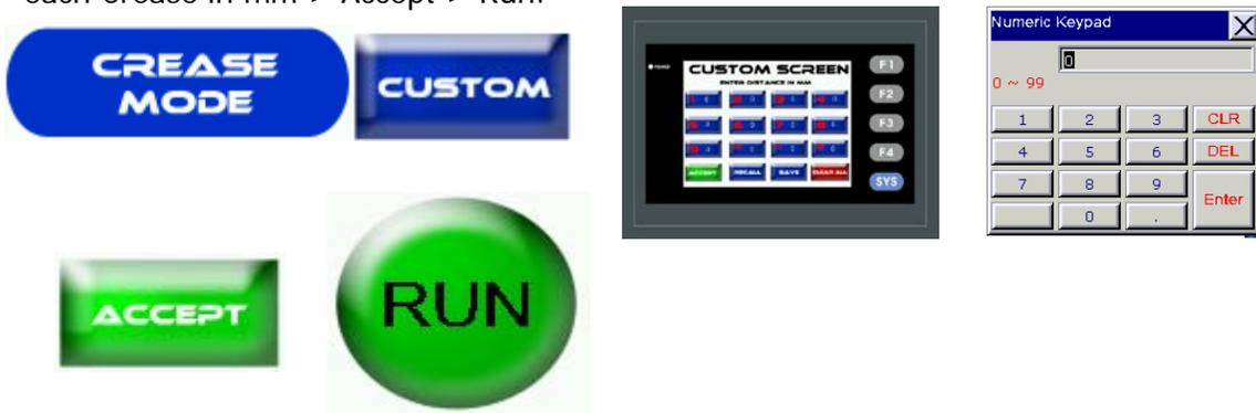
**Saving Custom Crease Jobs:** Press the Crease Mode Button > Custom > Enter In Distance For each Crease in mm > Save > Select Position to save in 1, 2, 3, or 4.
