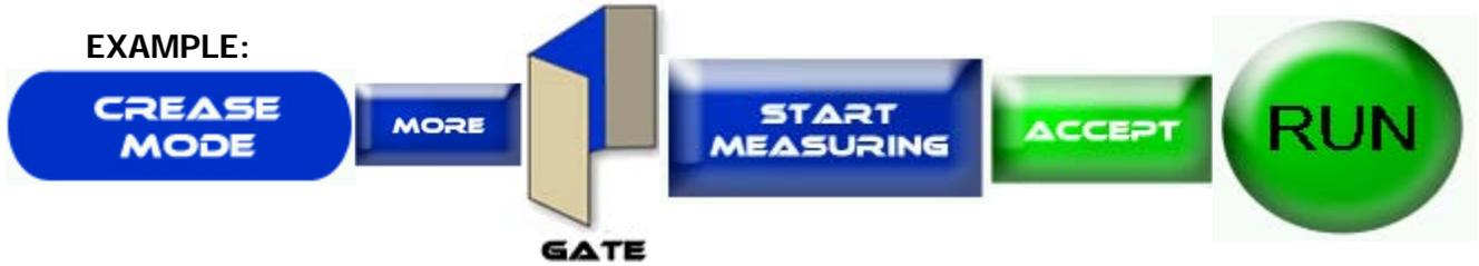
**Double Gate Fold:** Press the Crease Mode Button > More > Double Gate > Start Measuring > Physically Run a sheet through the machine for the sensor to measure > Accept > Run.
