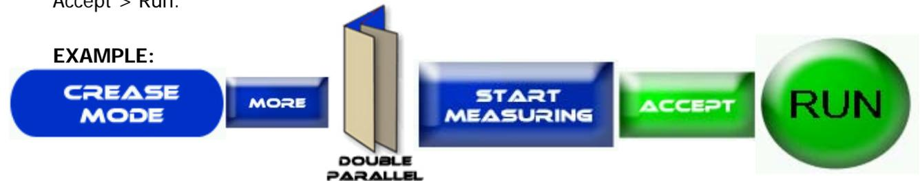
**Perfect Bind Double Hinge:** Press the Crease Mode Button > More > Perfect Binding Score > Enter The Book Thickness > Double Hinge > Start Measuring > Physically Run a sheet through the machine for the sensor to measure > Accept > Run.
