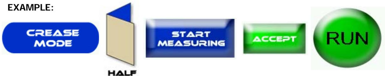
**Tri-Fold:** Press the Crease Mode Button > Tri-Fold > Start Measuring > Physically Run a sheet through the machine for the sensor to measure > Accept > Run.
