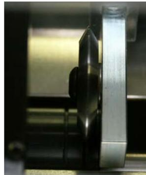
Position your score blade as desired. Scores should be made so that the blade runs on the side of the sheet that will be on the outside of the finished fold. Scores may be made on the EZ CREASER in three different ways using the different grooves on the lower score assembly.
