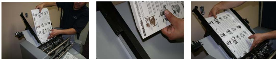
The better the spacing between the sheets and cleaner the fanning of the stack, the more efficient the feeder will perform.
