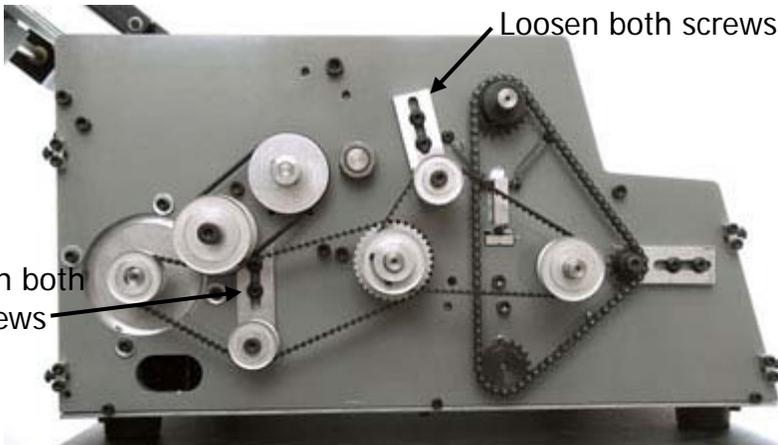
The shaft should not be able to move side to side. With both drive belts in Position, re-tension the belt idlers and tighten while applying constant firm pressure on the belts by pushing down on the tops of the brackets with the large T-handle wrench supplied. Replace covers. Align upper assemblies accordingly.
