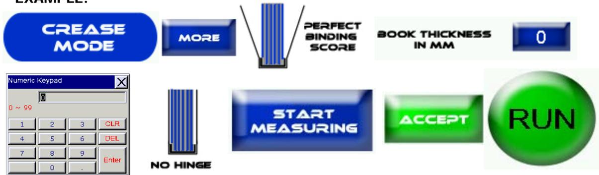
**Custom Crease Job:** Press the Crease Mode Button > Custom > Enter In Distance For each Crease in mm > Accept > Run.
