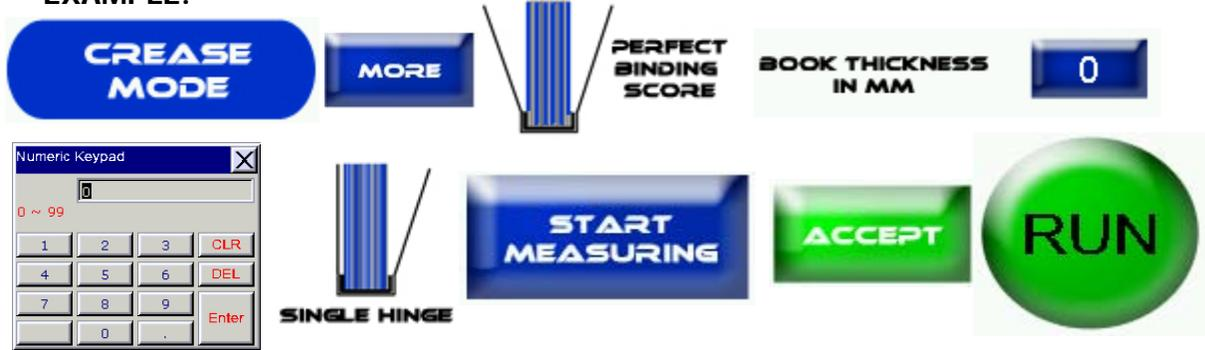
**Perfect Bind No Hinge:** Press the Crease Mode Button > More > Perfect Binding Score > Enter The Book Thickness > No Hinge > Start Measuring > Physically Run a sheet through the machine for the sensor to measure > Accept > Run.
