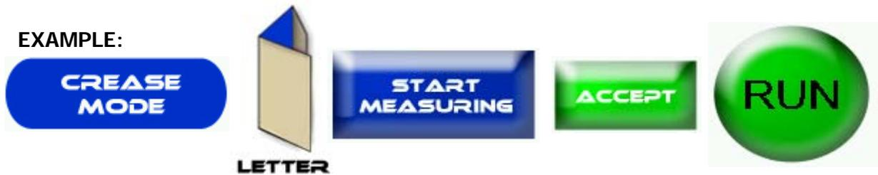
**Roll Fold:** Press the Crease Mode Button > More > Roll > Start Measuring > Physically Run a sheet through the machine for the sensor to measure > Accept > Run.
