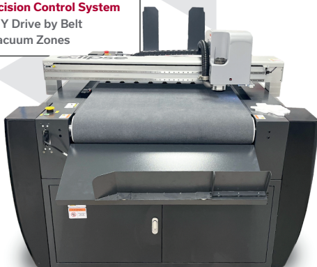
Precision Aluminum Table With multiple vacuum zone system for accurate material hold down.
