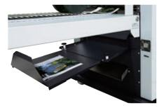
Errored sets are rejected to the reject tray so that only correct booklets are delivered to the conveyor.
