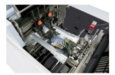
The wire feeding sensor alerts when the wire spool is nearly empty or jamming, and stops the system to eliminate non-stitched booklets. Up to 48 sheets of normal paper (64 gsm / 50lb. offset) can be stitched or up to 24 sheets of normal paper (64 gsm / 50lb. offset) can be stitched and folded. The stitching position and distance are automatically set up for the input size.
